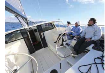
Above: cockpit benches are well protected under the carbon canopy. High bulwarks make comfortable backrests to sit out on the side decks
