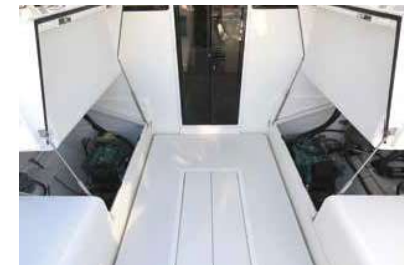
Above: twin engines are fitted under the cockpit benches. These are good for manoeuvring and keeping noise out of the interior
