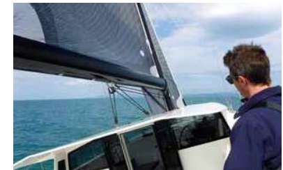
Above: clear sightlines over the low coachroof and through the decksaloon windows. Note the simple, three-point mainsheet system
